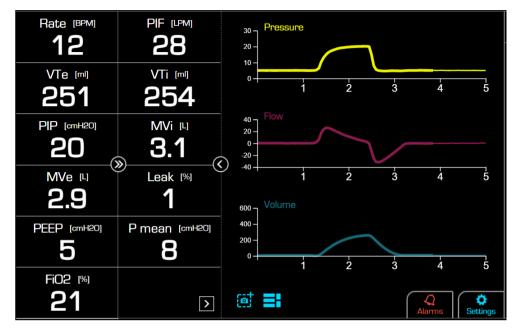
The user can scroll between 3 columns of secondary parameters with the arrow at the bottom:
