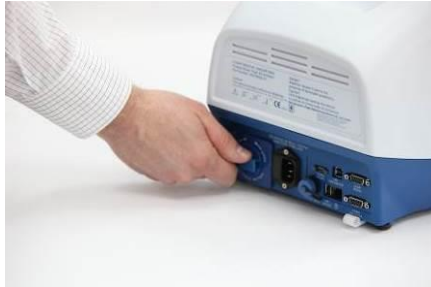
Figure 6 – Installing the Detachable Battery
