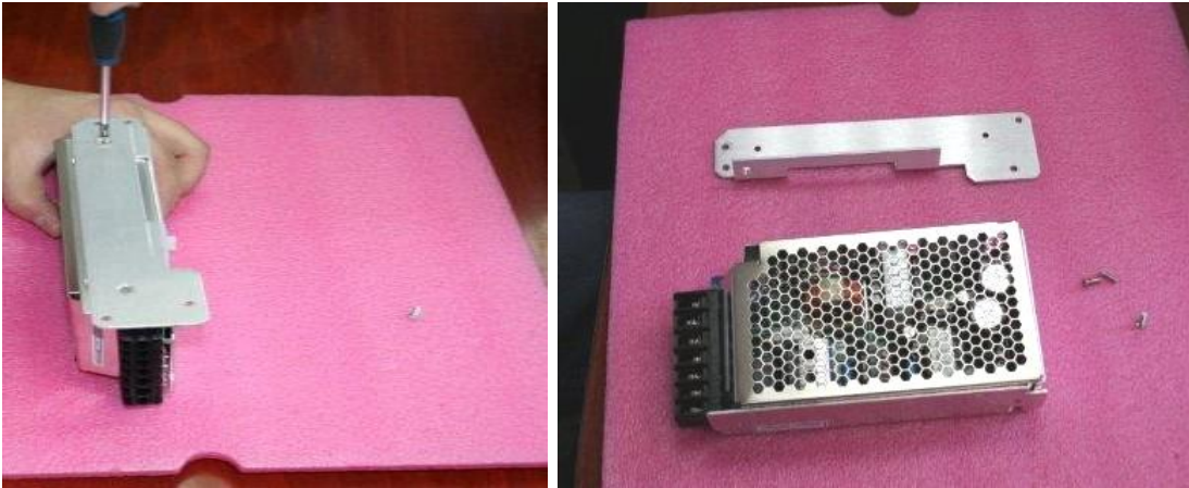
Figure 25 – Detaching the Power Supply from Its Bracket
