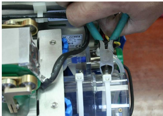
Figure 44 - Cutting the Cable Ties
