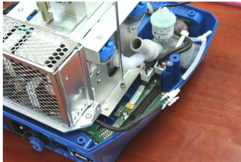
Figure 49 – Detaching the Manifold Base
