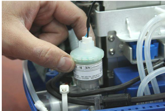
Figure 52 – Removing the Oxygen Sensor
