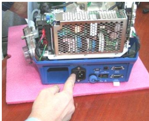
Figure 70 – Connecting the Fuse
