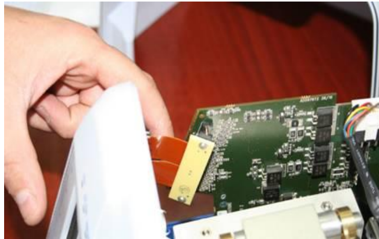
Figure 30 – Flat Flex Cable going to P16
