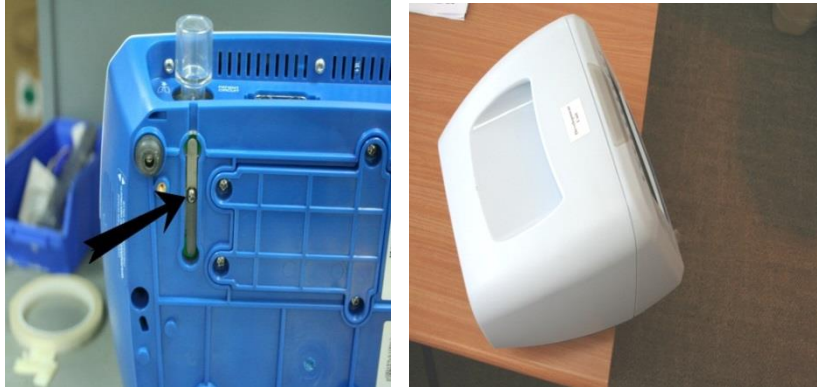
Figure 72 –Adjusting the Pressure Relief Valve
