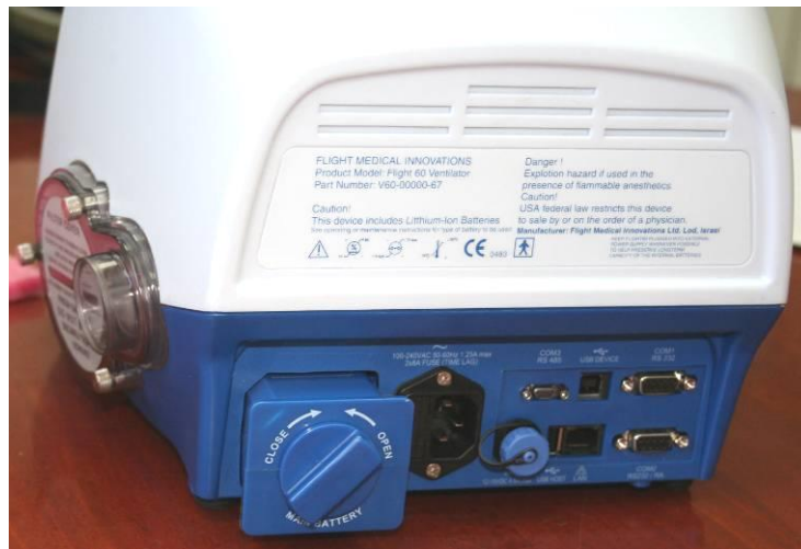
Figure 8 – Removing the Detachable (Main) Battery
