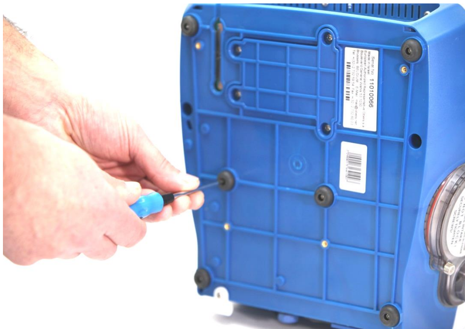
Figure 71 – Removing a Rubber Bumper
