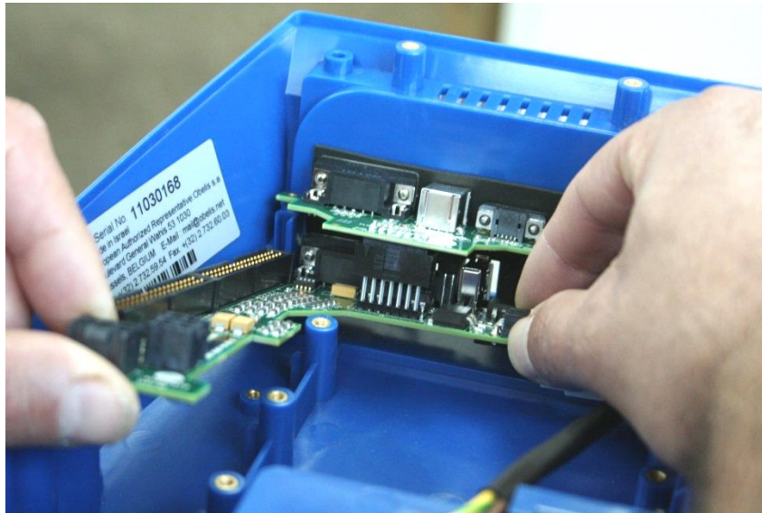
Figure 67 – Removing the Lower Board and D-type Board
