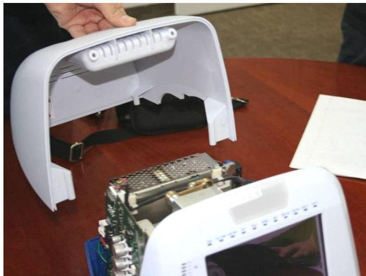
Figure 13 – Removing the Ventilator Cover
