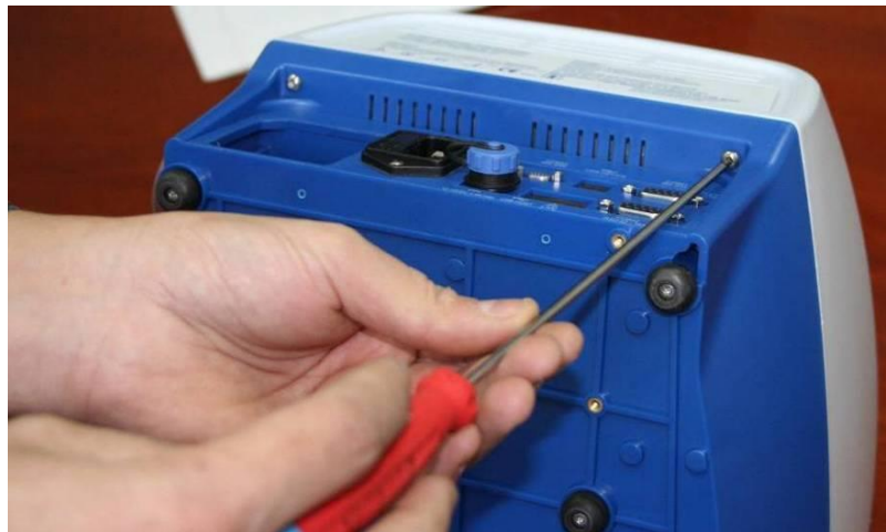
Figure 9 – Removing Back Screws
