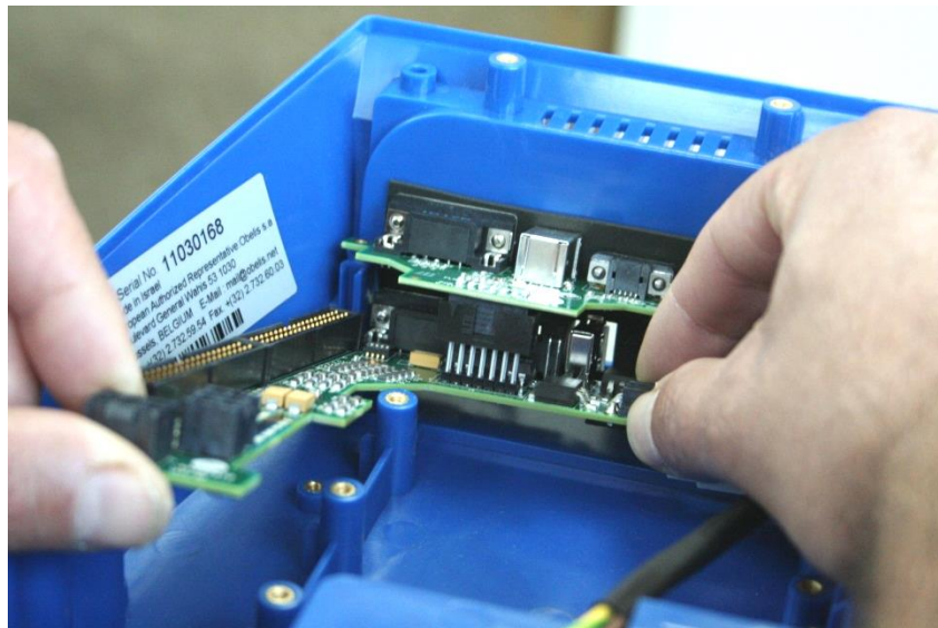
Figure 39 – Removing the Lower Board and D-type Board
