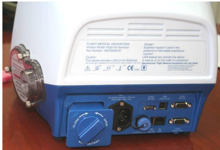
Figure 6 – Removing the Detachable (Main) Battery
