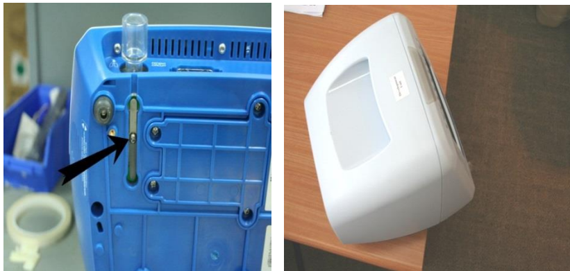
Figure 42 –Adjusting the Pressure Relief Valve
