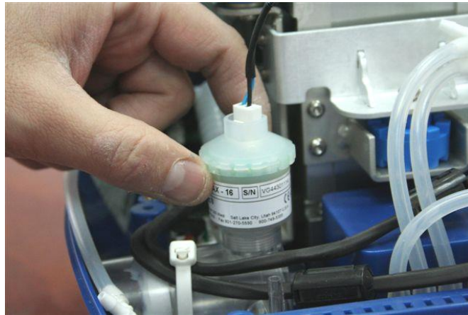
Figure 30 – Removing the Oxygen Sensor
