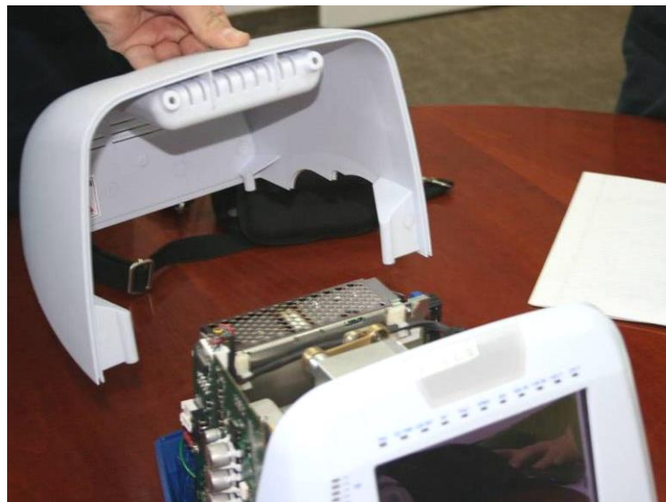
Figure 11 – Removing the Ventilator Cover
