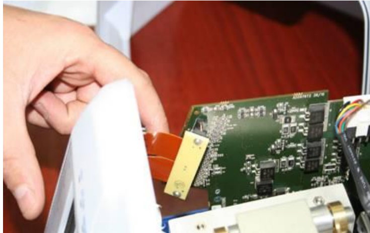
Figure 30 – Flat Flex Cable going to P16
