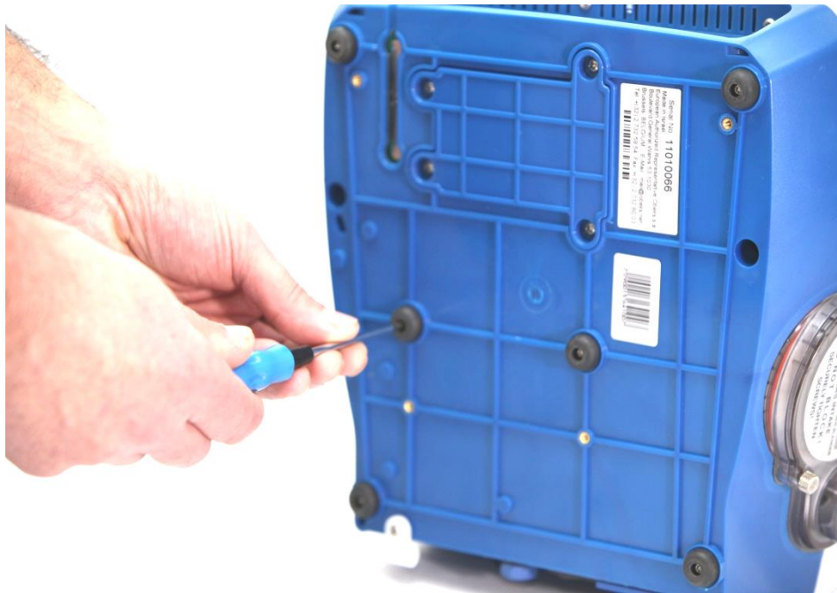
Figure 71 – Removing a Rubber Bumper
