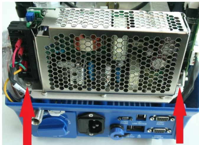
Figure 24 –Power-Supply Bracket screws
