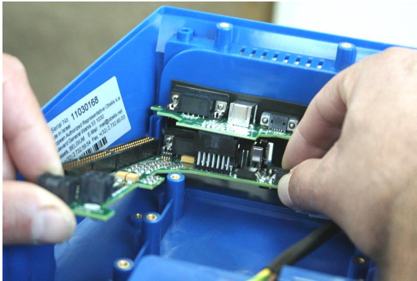
Figure 67 – Removing the Lower Board and D-type Board
