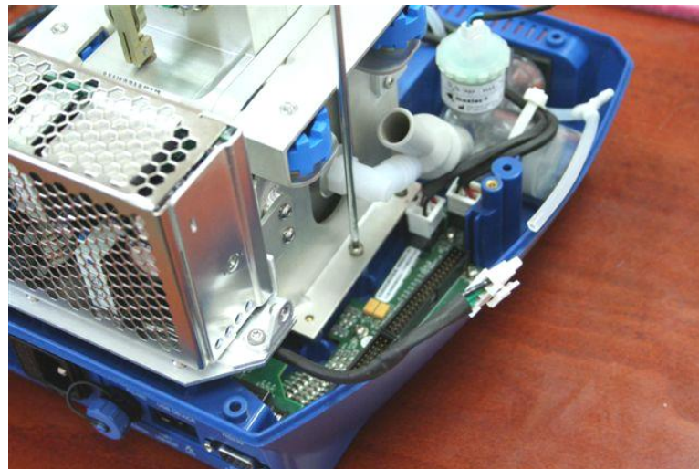
Figure 49 – Detaching the Manifold Base
