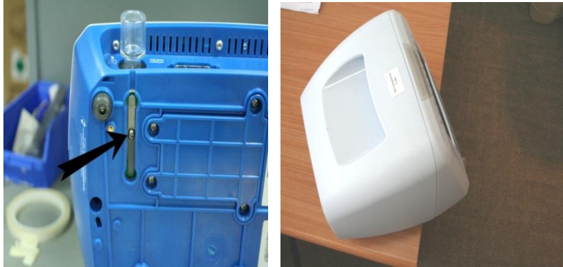
Figure 72 –Adjusting the Pressure Relief Valve
