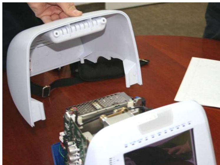
Figure 13 – Removing the Ventilator Cover
