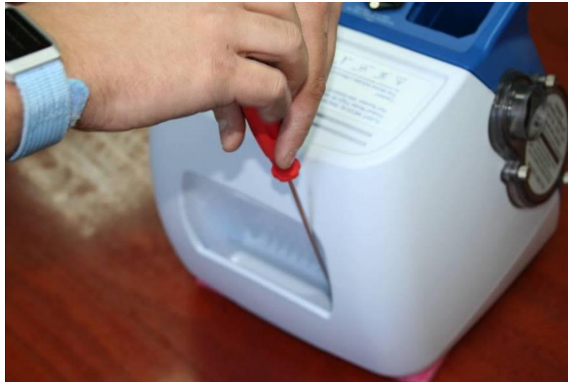
Figure 10 – Removing Screws Inside Handle
