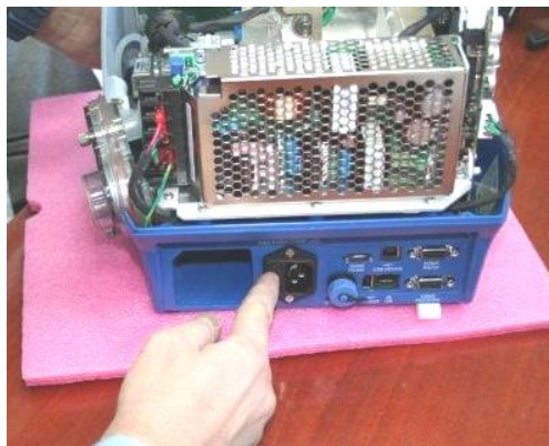
Figure 70 – Connecting the Fuse
