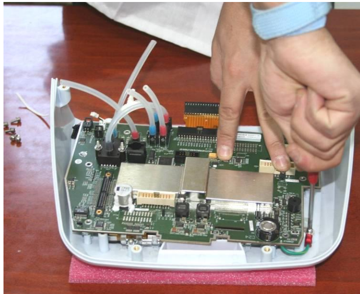
Figure 39 – Detaching the Grounding Screw
