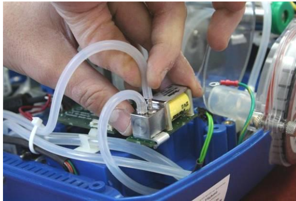
Figure 36 – Removing the Silicon Tubes
