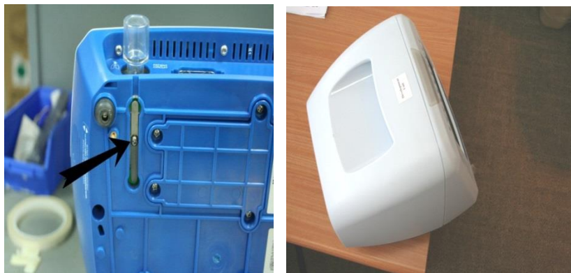
Figure 42 –Adjusting the Pressure Relief Valve
